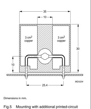
Fig.5 Mounting with additional printed-circuit board for heat sink purposes.
