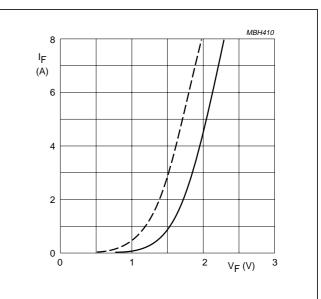
Dotted line:  $T_j = 150 \,^{\circ}\text{C}$ . Solid line:  $T_j = 25 \,^{\circ}\text{C}$ .
